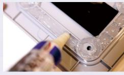
2 Fill the edge groove with enough silicon adhesive to apply the entire circumference
