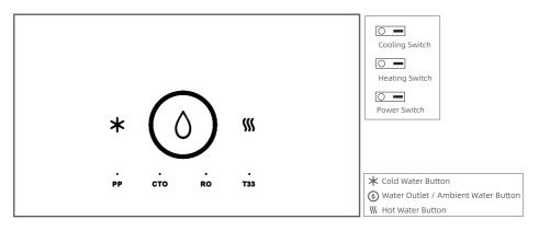
•Heating switch on (switch position will be from "O" to "-".), the machine will start heating.
