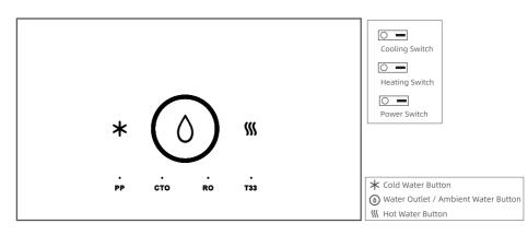
•Press Water Outlet / Ambient Water Button ③ on control panel, and you will get ambient water (there will be green circling light around "water outlet" button ④).
